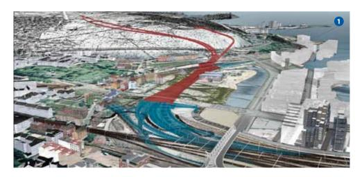
Norway's longest railway tunnel will be constructed using tunnel boring machines, as well as traditional drill and blast methods. This is the first time that tunnel boring machines will be used in Norway to build a railway tunnel.
