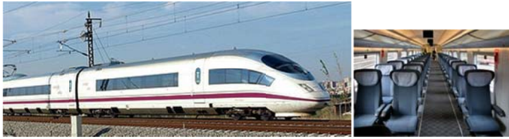
Figure 15. Siemens Velaro (AVE S-103) high speed train 1+2 and 2+2 seating. Standard body width. Total capacity 536 seats (8 cars). Commercial speed 350 km/h
